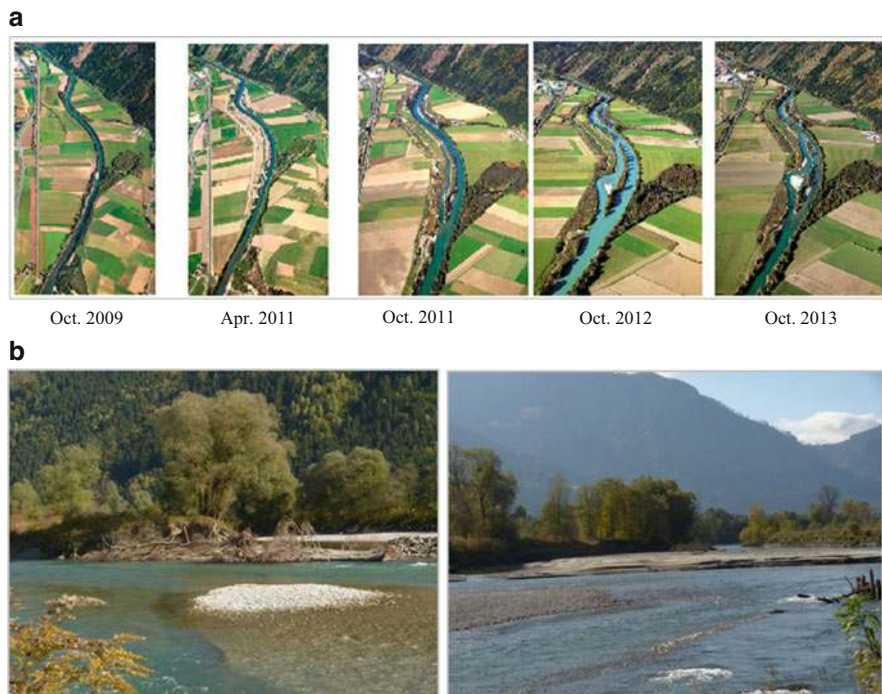
Fig. 15.2 (a) “Self-development” of the Drava river course (at Obergottesfeld/Carinthia) after removing bank protection and initial channel creation (LIFE project: Life vein-Upper Drau River) (photographs: Herbert Mandler, © Amt der Kärntner Landesregierung). (b) Morpho-dynamic processes supported the development of key aquatic habitat types (sediment bars and islands; woody structures along the riparian corridor of the Upper River Drava) (photographs: Susanne Muhar)
