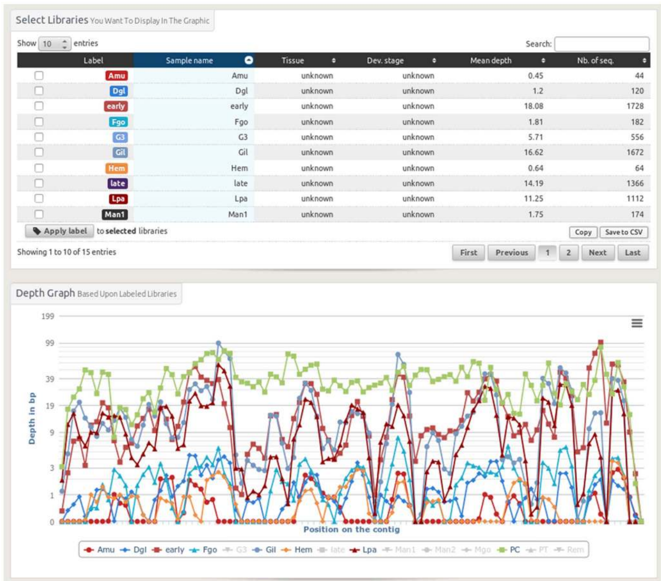
Figure 6. The contig depth view enables to visualise the coverage of the reads of the different libraries on a given contig. Each library has a defined colour in the table and the same one on the graphic. It is possible to modify the graphical layout by averaging different library depths. This is typically to be used when you work with replicates. doi:10.1371/journal.pone.0096821.g006
