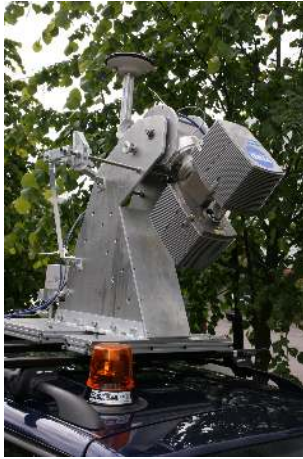
Figure 2. The ROAMER instrumentation on its first field run. The scanner is tilted to the backward direction.
