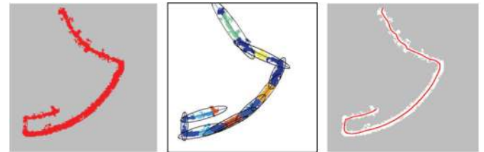
Fig. 8. Road centerline extraction based on GMM. (a) Road region. (b) Long axes of GMM. (c) Axes adjusted by SCMS.
