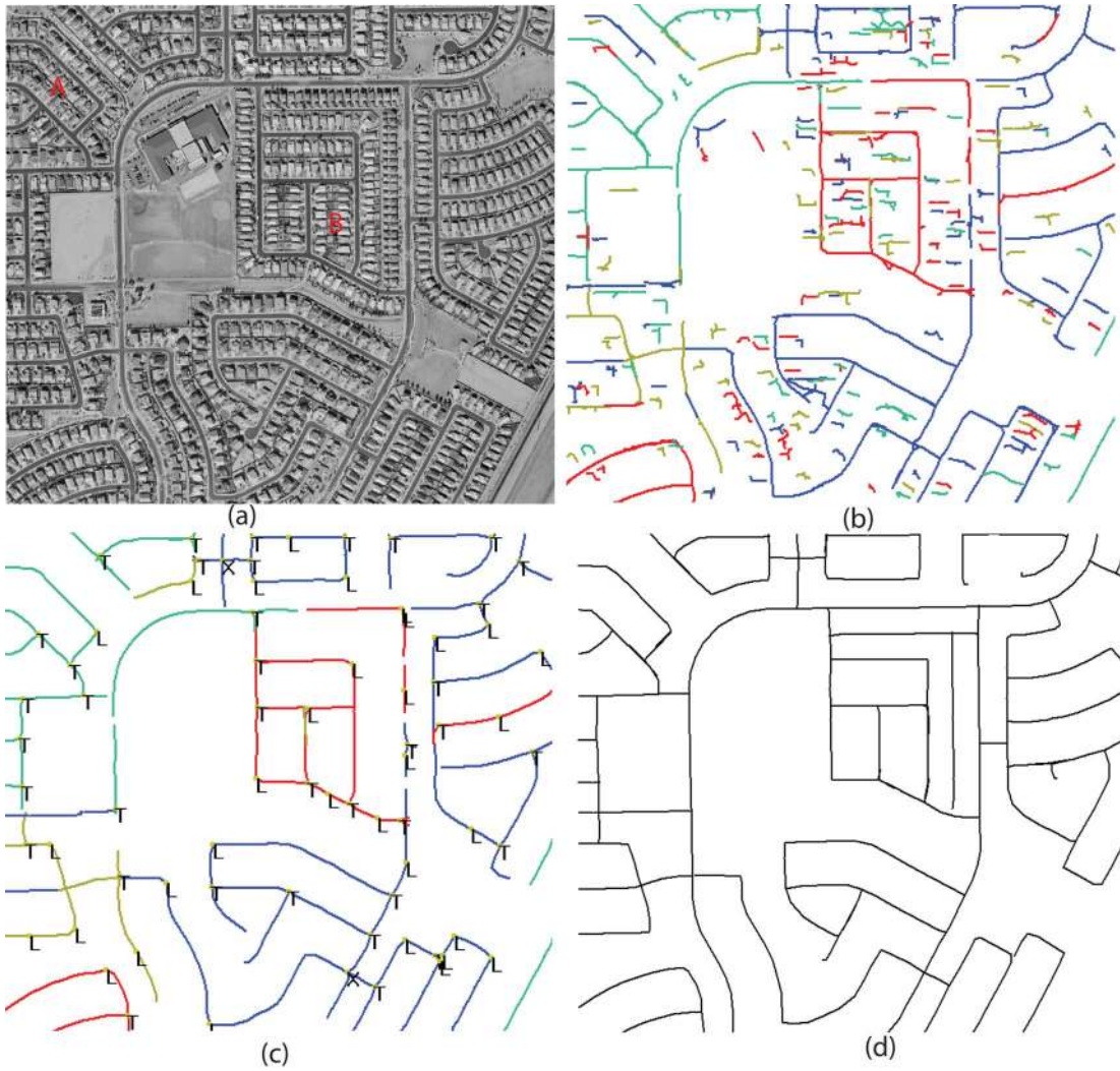
Fig. 16. Road network detection based on automatic seeding. (a) Original image. (b) Inscribed line of road extraction before the road tree was pruned. (c) Inscribed line of road extraction after the road tree was pruned. There are 30 L -shaped corners, 36 T -shaped intersections, and 2 X -shaped intersections. (d) Reference roads.
