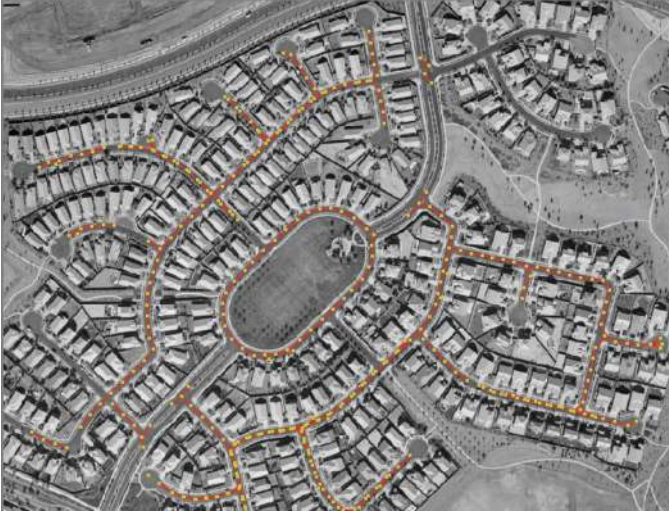
Fig. 12. Road inscribed line after road tree pruning based on the Gaussian model. It is obvious that some vertices on the road were also pruned.
