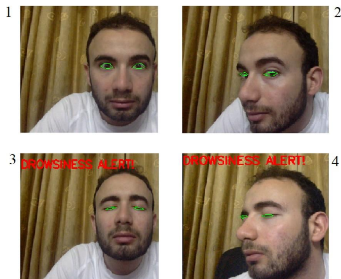
Fig. 7. Smart car-camera part for sleepy driver sequence diagram
