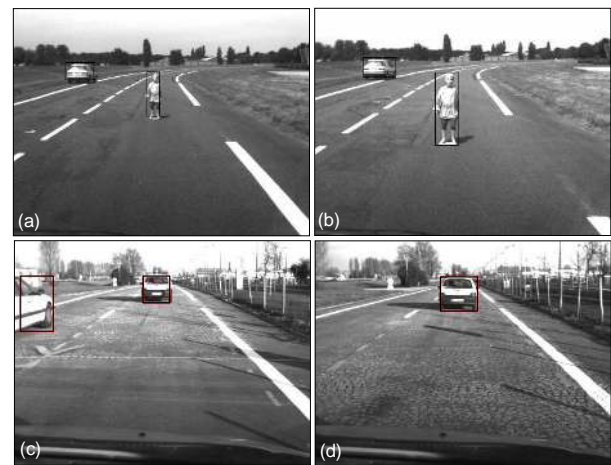
Fig. 11. Examples of bounding boxes around multiple objects: (a)(b) a car and a pedestrian; (c)(d) two cars on a paved road, which is a typical periodic noisy texture.
