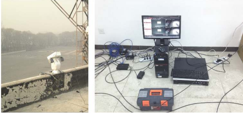
FIGURE 1: Road surface images acquisition system.
