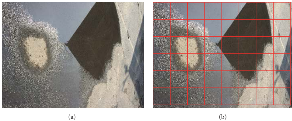
FIGURE 17: Image test results of hybrid road surface (from the mobile image). (a) Image of hybrid road surface state. (b) Image blocks.
