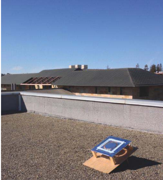
Figure 2 – Outdoor test of a daytime radiative cooling surface. A test stand that insulates and minimizes parasitic heat gain is essential to maximize performance. A unique feature of radiative cooling experiments is the need to perform tests outdoors.
