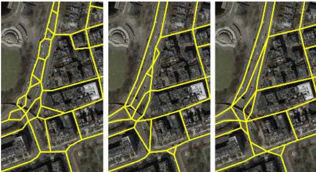
Figure 9. Tradeoff between error rate and recall in a small crop from Boston as we increase the threshold for our segmentation approach. The junction metric error rates in the crop from left to right are 18%, 13%, and 8%. The map with 18% error is too noisy to be useful.
