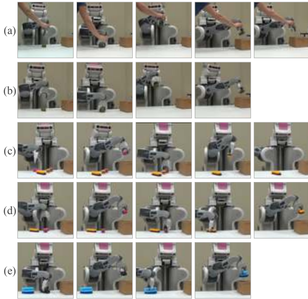
Fig. 4: (a) Demonstration of the manipulation procedure for picking up a small block and placing it in a large box. (b-c) Execution of the looping program in the original scene it was demonstrated and a new scene with more objects. (d-e) Execution of the looping program with different object matching condition thresholds.
