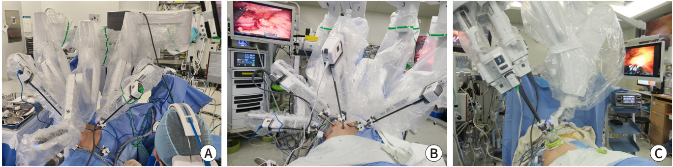
Fig. 1. Da Vinci robot surgical systems, (A) X system, (B) Xi system, and (C) SP system. Constant improvement of the technology has expanded the use of robot-assisted surgery in colorectal diseases.
