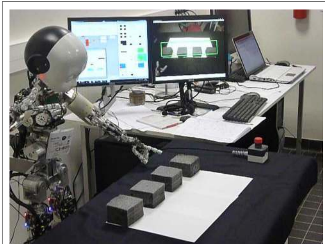
FIGURE 3 | iCub robot performing Experiment 3. The robot chooses among four cubes on a table. The left screen tracks simulated activity in the neural-network model. The right screen shows the perception of the robot.
