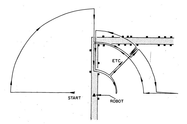
In this figure, we have superimposed the eye's scan-path over a map of the territory in front of the robot. The scan-path is the locus of the center point of the robot's visual field.
