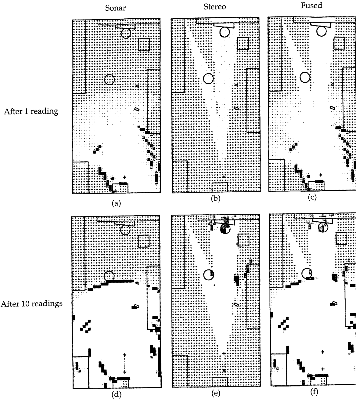
FIGURE 9 Fusion of Sonar and Stereo. Fusion is trivial in the evidence grid framework: we simply add the log odds of corresponding cells. The “+” marks the location of the robot, which moved in a straight line taking readings at evenly spaced intervals. From [Matthies-Elfes88], [Elfes-Matthies87], and [Moravec88]
