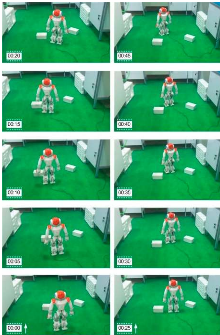
Figure 6. The path traversed by the Nao humanoid robot using the fuzzy synthetic potential field method (see the video of the robot’s movement).
