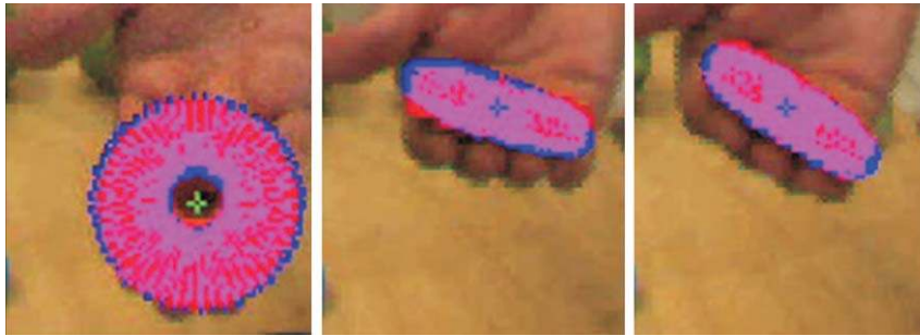
Fig. 13. Pose estimation of a disc with a fixed camera.
