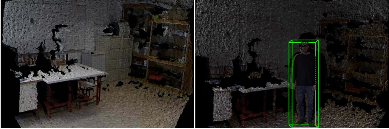
Figure 4. People detection algorithm. The figure on the left was captured when there were no people on it, the second one detected one person and created a bounding box over it.
