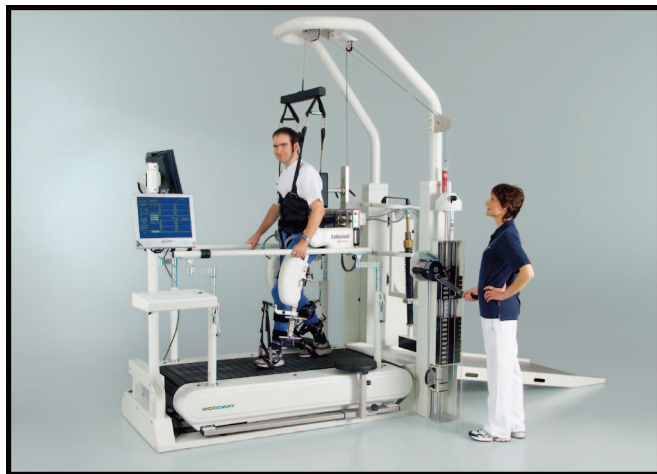
Figure 1. The driven gait orthosis (DGO) (Lokomat) used during robotic-assisted treadmill training. Image used with permission from Hocoma AG Inc, Zurich, Switzerland.
