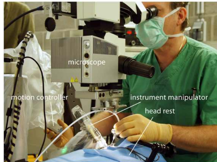
Fig 1. Surgical set-up used to operate the animals. The Preceyes micromanipulator is positioned for this intervention for the right eye of a pig. The motion controller is handled by the surgeon, from the temporal side of the eye within the surgical field and well within reach of the eye itself. The surgeon remains in his standard operating room position. In his left hand, he is holding a handheld endoilluminator (free hand).
