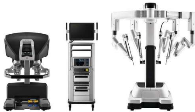
Figure 3 The da Vinci Surgical System ® (Intuitive Surgical, Sunnyvale, California) robot. Image courtesy of Intuitive Surgical Inc. da Vinci Si System with single-site instrumentation. Surgeon console, surgeon, da Vinci ® Si patient cart with Single-Site ™ instruments. Available from: https://www.intuitivesurgical.com/company/media/images/singlesite.php . Accessed September 22, 2019. Copyright © 2019 Intuitive Surgical, Inc. 64
