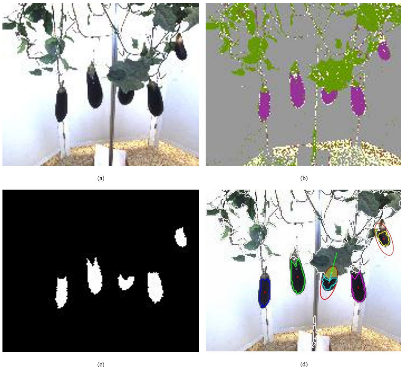
FIGURE 12. Experimental results - Test 4: a) registered RGB image; b) pixel-based classification map; c) ground truth data; d) output of the aubergine class. The red asterisks represent the centroids estimated from the detected aubergine blobs, the irregular colored lines show the contours of the detected aubergine blobs, the white irregular lines correspond to the contours of the detected leaf blobs, the red ellipse indicates the model template superimposed over the occluded blob, and the green line represents the direction vector that the robotic arm follows to brush the leaves aside and remove the occlusion.
