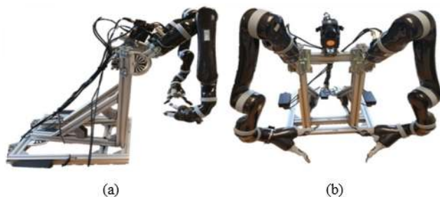
FIGURE 1. Prototype of the dual-arm harvester robot. a) lateral view b) front view.
