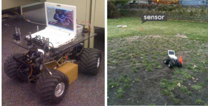
Figure 13: Left: Cyclops robotic platform developed for data muling. Right: A data mule system together with sensors.
