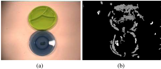
Figure 6: (a) An image of textureless/transparent/reflective objects. (b) Depths estimated by our stereo system. The grayscale value indicates the depth (darker being closer to the camera). Black represents areas where stereo vision failed to return a depth estimate.
