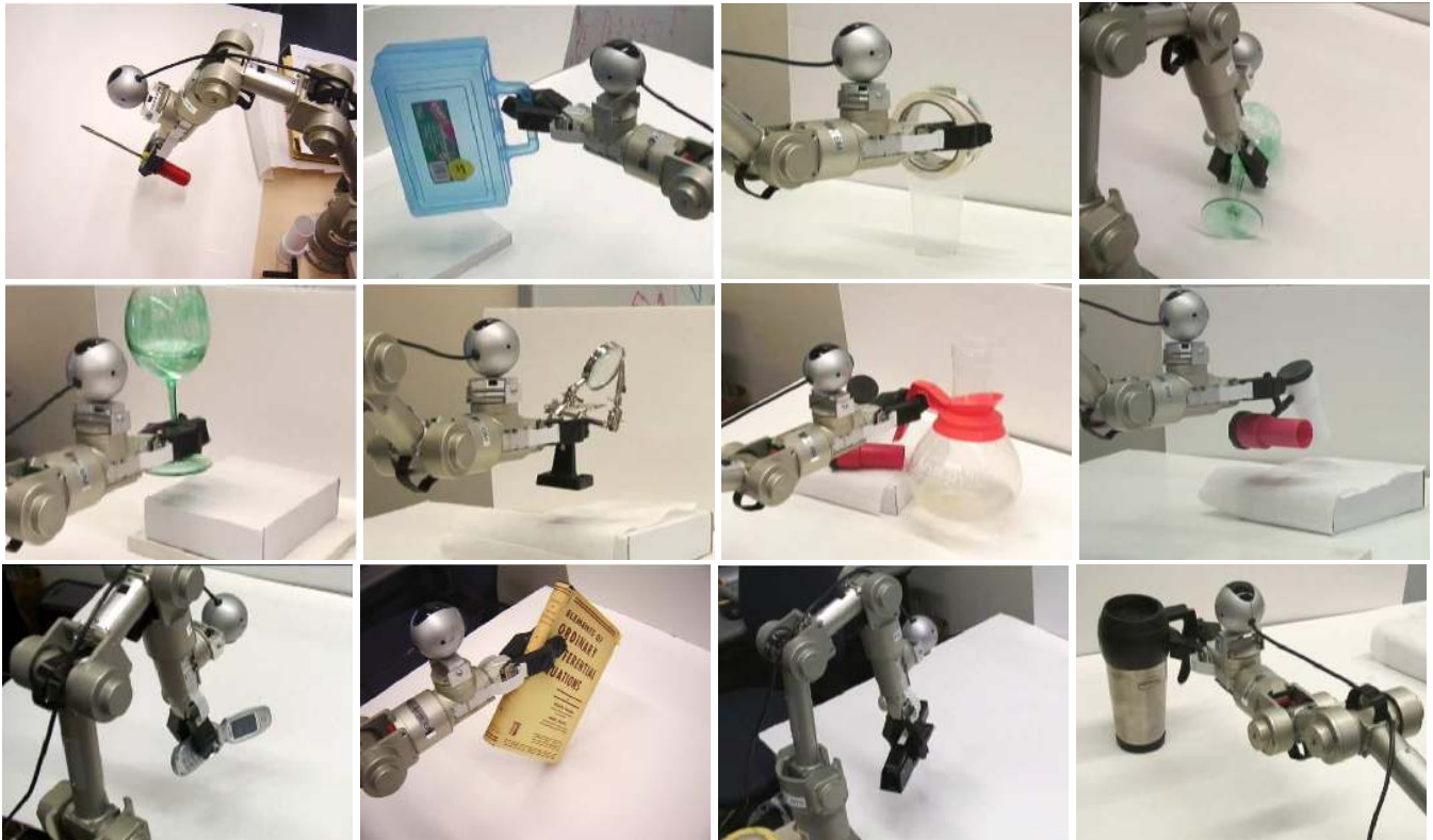
Figure 11: The robotic arm picking up various objects: screwdriver, box, tape-roll, wine glass, a solder tool holder, coffee pot, powerhorn, cellphone, book, stapler and coffee mug. (See Section 6.2.)
