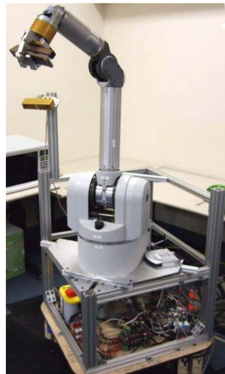
Figure 10: STAIR 2 platform. This robot is equipped with 7-dof Barrett arm and three-fingered hand.
