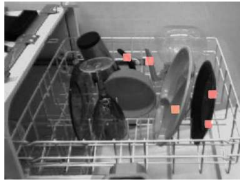
Figure 13: Grasping point detection for objects in a dishwasher. (Only the points in top five grasping regions are shown.)
