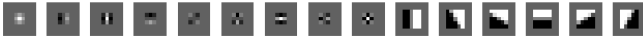
Figure 5: Examples of different edge and texture filters (9 Laws’ masks and 6 oriented edge filters) used to calculate the features.
