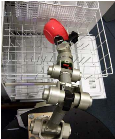
Figure 15: Dishwasher experiments: Failure case. For some configurations of certain objects, it is impossible for our 5-dof robotic arm to grasp it (even if a human were controlling the arm).
