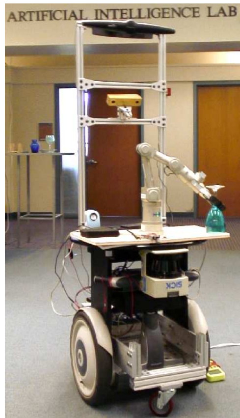
Figure 9: STAIR 1 platform. This robot is equipped with a 5-dof arm and a parallel plate gripper.
