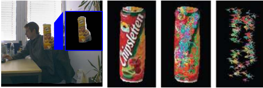
Fig. 6. Spatial segmentation for object learning (left), side view of an object, detected feature points and corresponding feature point cloud (right three images)
