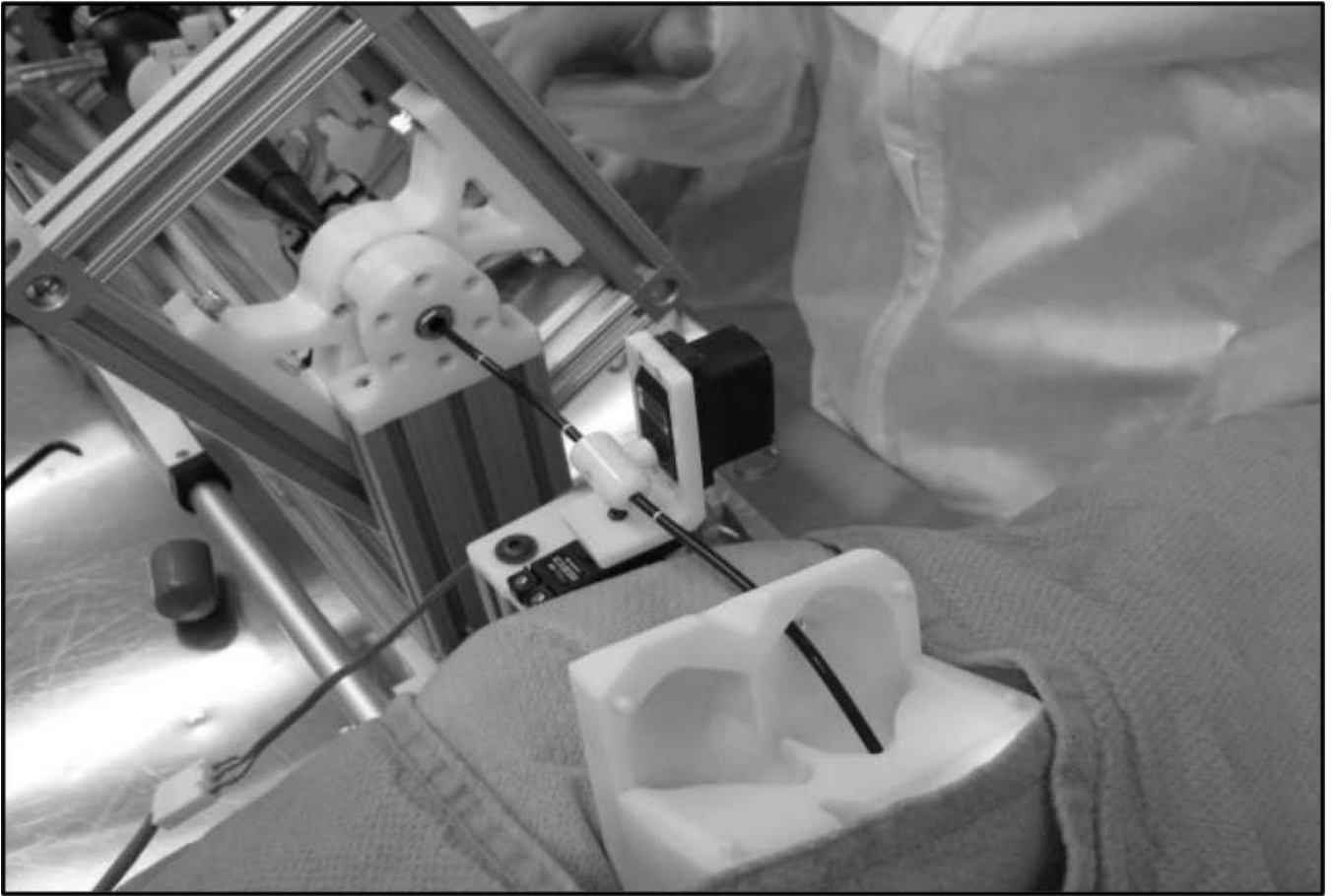
Fig. 11. Experimental setup, showing robotic endoscope and 3D ventricular model.
