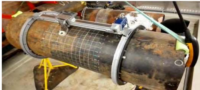
(a) Exhumed pipe on which internal and external measurements were performed.
