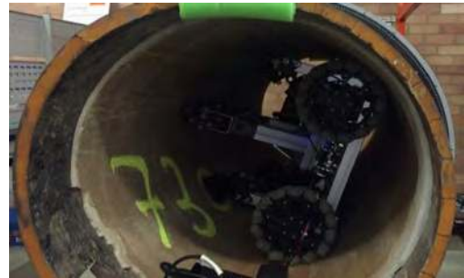
(b) Pipe assessment robot performing internal measurements.
