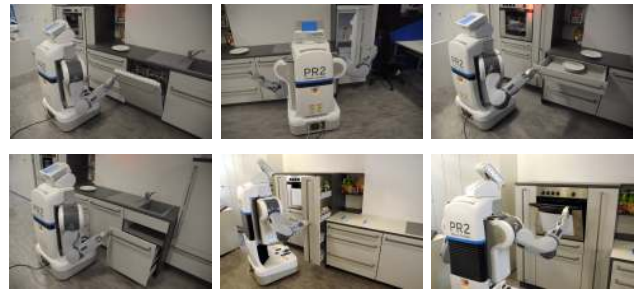
Fig. 5. The PR2 opening different containers using the same controller without knowledge of the mechanism but only of the handle position.
