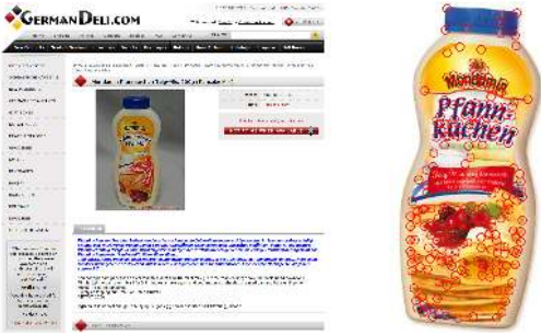
Fig. 3. Bottle of pancake mix from GermanDeli.com (left), and the extracted features to recognize the object (right).
