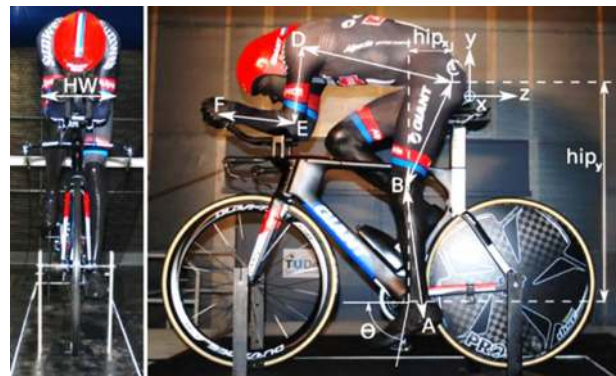
Fig. 5 Cyclist mannequin in front (left) and side view (right) with indication of characteristic dimensions
