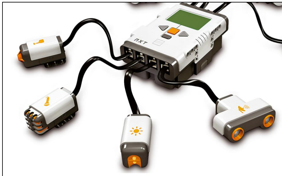
Figure 3. The NXT sensors. The default settings used for the test programs on the NXT requires the touch sensor to be connected to port 1; the sound sensor to be connected to port 2; the light sensor to be connected to port 3 and the ultrasonic sensor to be connected to ports 4 on the NXT brick.
