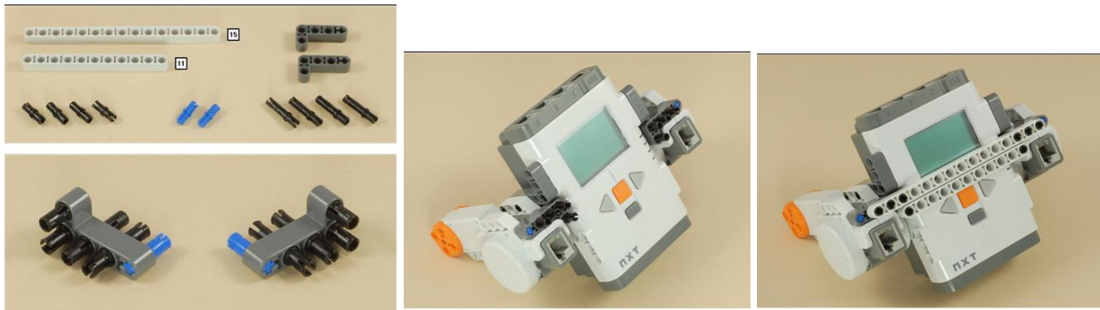
Figure 4. Example of a building instruction. The parts needed are shown first then the assembly of each part to the main structure is shown.
