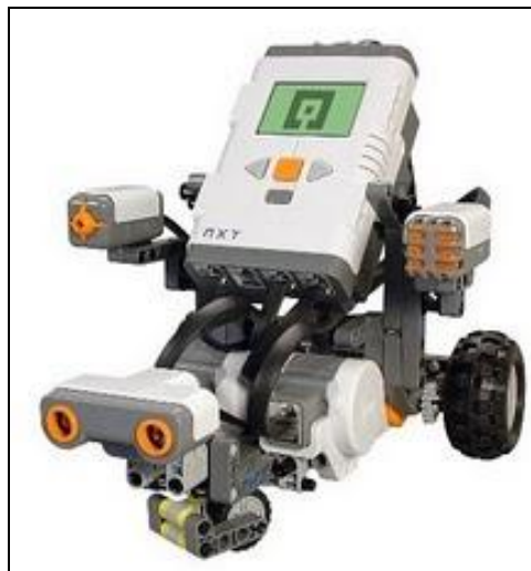
Figure 5. An illustration of a Taskbot model with its ultrasonic, touch, and sound sensor attachments.
