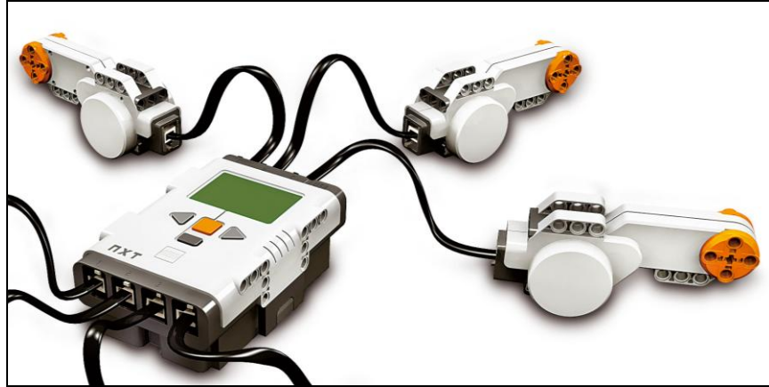
Figure 2. NXT motors with embedded rotation sensor connected to its respective ports on the NXT brick using cables that resemble telephone cables.
