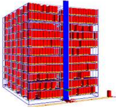
Figure 7: A crane-based multi-deep compact storage system (De Koster et al. 2008)
