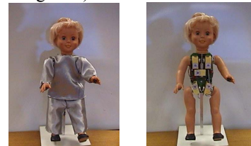
Figure 1 The robot Robota. The figure on the right shows the 'undressed' version revealing the robotic parts that control its movement
