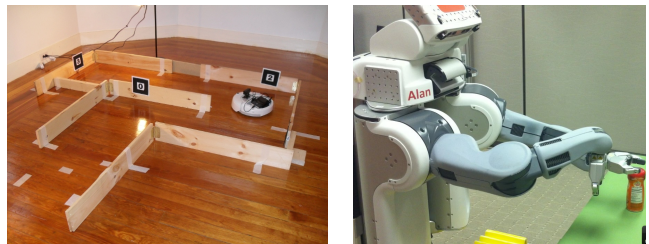
Fig. 3: Two different remote labs currently under development. The first depicts an iRobot Create learning to navigate a maze. The second contains a PR2 that can manipulate objects on a table.
