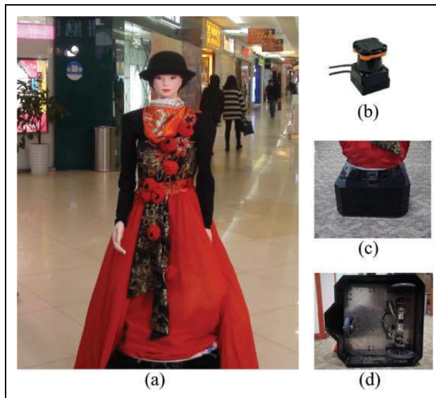
Figure 2. (a) KeJia robot. (b) Laser scanner. (c) Robot chassis. (d) Differential wheels.
