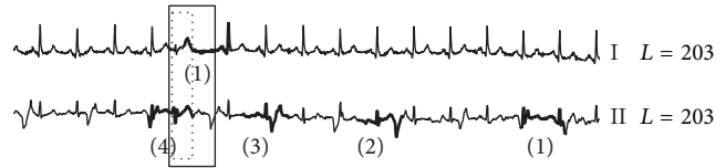
FIGURE 19: Anomaly detection result of the INCARTDB04 dataset by BitClusterDiscord algorithm with L = 203 .
