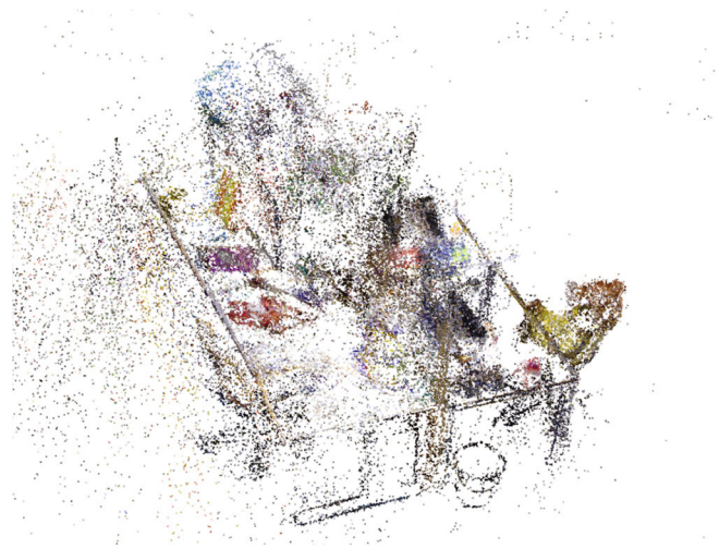
Fig. 9 Ego-motion estimation and mapping results for our proposed algorithm on the fr3/long_office sequence from the TUM RGB-D dataset.
