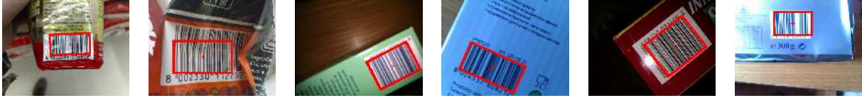
Fig. 1. Examples showing the barcode bounding boxes detected by the proposed method for arbitrary rotated 1D barcodes appearing in camera captured images; the detected bounding boxes are correct even when the barcodes are twisted, occluded or partially illegible due to reflections.
