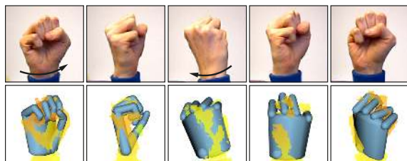
Figure 22: Our algorithm relies on the presence of salient geometric features in the depth map. Challenging sequences like a rotating fist lack such features when acquired with current commodity depth sensors, which can result in loss of tracking.
