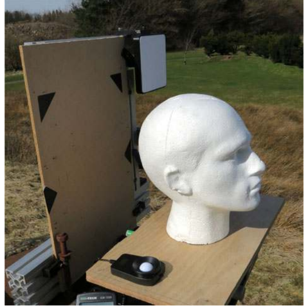
Fig. 1. Photograph showing the polystyrene head used for the experiments described here and calibration targets, including the Spectralon panel (top right corner of the fiberboard).
