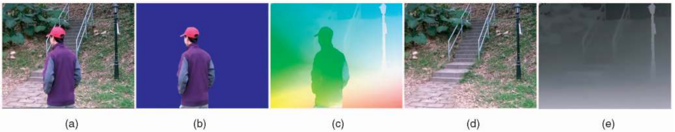
Fig. 14. “Stair” example. (a) One input frame. (b) The extracted foreground image. (c) The computed optical flow map. (d) The estimated background image. (e) The recovered background depth map.
