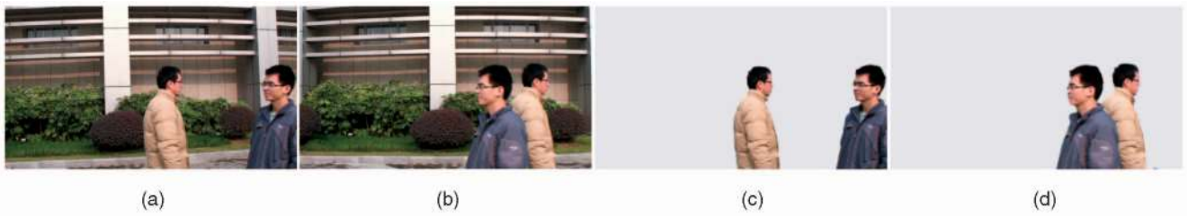
Fig. 22. "Two-Men" example. (a)-(b) Two selected frames. (c)-(d) Extracted foreground images.
