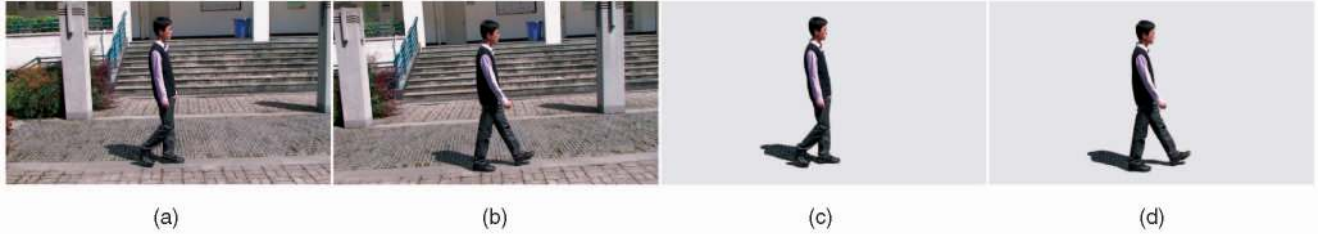
Fig. 23. "Shadow" example. (a)-(b) Selected frames. (c)-(d) The extracted foreground images. The shadow is recognized as part of the foreground.
