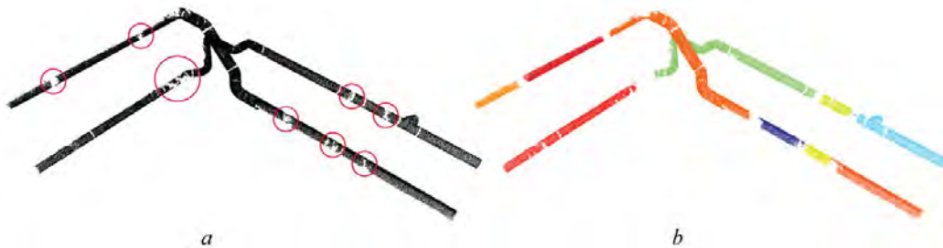
Figure 6. a) Ground truth segmentation of two composite pipes. The red circles show areas with missing data due to occlusions. b) The over segmentation resulting from missing data.
