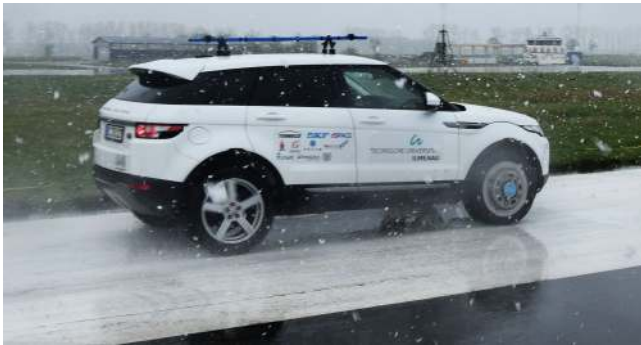
Fig. 8. Vehicle demonstrator on the low- \mu road surface during testing in severe weather conditions. Represented road section is covered with the special friction layer, which is continuously wet with water sprinklers.
