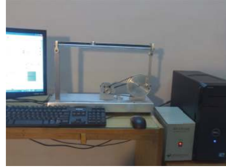
FIGURE 9: Experimental setup of the ball and beam equipped via GoogolTech GBB1004.
