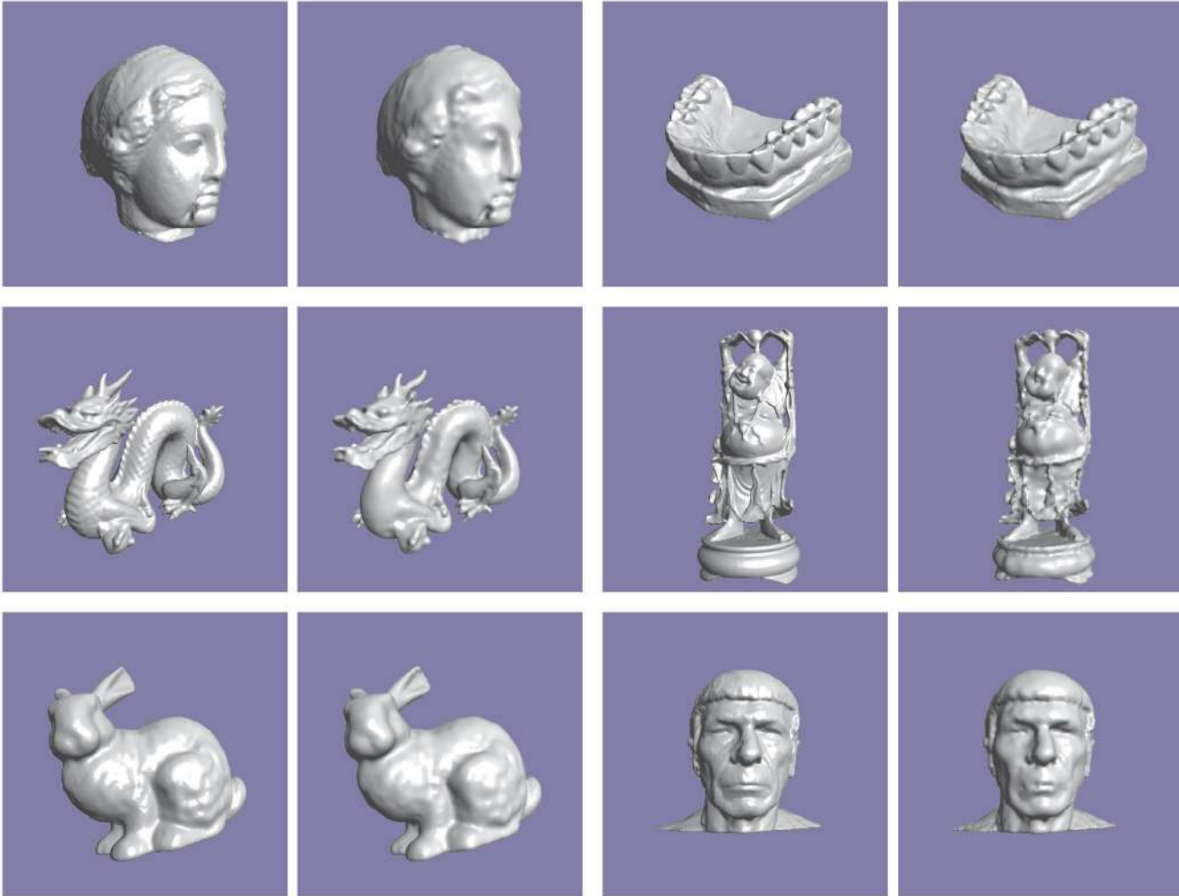
Fig. 7. Six large scanned polygonal models: intermediate volumetric representations (left images of pairs) and final implicit surfaces (right images of pairs) from our algorithm.
