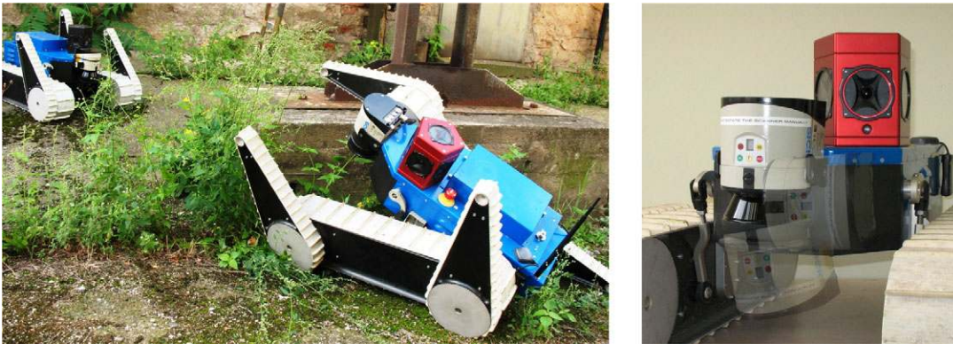
Figure 1. Picture of two USAR UGVs used for experimental evaluation (FP7-ICT-247870 NIFTi project) and a detail of the sensor setup (a PointGrey Ladybug 3 omnicaamera and a rotating SICK LMS-151 laser rangefinder). See Section 3.1 for more details.
