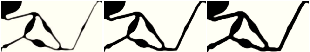
Figure 4. Three threshold projections, eroded, intermediate and dilated, obtained with thresholds \eta = 0.6, 0.5 and \eta = 0.4 , respectively. The design is obtained using large displacements robust optimisation formulation with threshold \eta \in \mathcal{U}[0.3, 0.7] and volume constraint 30% of the original volume imposed on the dilated projection at \eta = 0.3 . The objective is E[c] = -7.85 \mu\text{m} , the standard deviation is \text{STD}[c] = 1.0 , the number of the integration points is 2, and the projection parameter is \beta = 32 . The objective expectation and standard deviation, computed with 31 integration points Kronrod-Patterson rule are E[c] = -8.43 and \text{STD}[c] = 5.83 .
