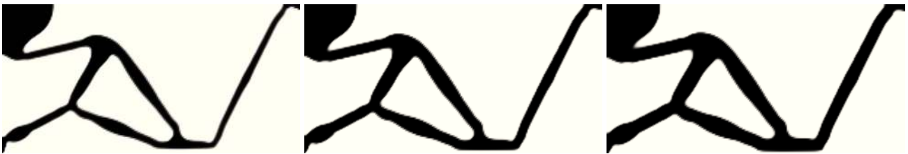
Figure 5. Three threshold projections, eroded, intermediate and dilated, obtained with thresholds \eta = 0.6, 0.5 and \eta = 0.4 , respectively. The design is obtained using large displacements robust optimisation formulation with threshold \eta \in \mathcal{U}[0.3, 0.7] and volume constraint 30% of the original volume imposed on the dilated projection at \eta = 0.3 . The objective is E[c] = -8.96 \mu\text{m} , the standard deviation is \text{STD}[c] = 5.80 , the number of the integration points is 31, and the projection parameter is \beta = 32 .
