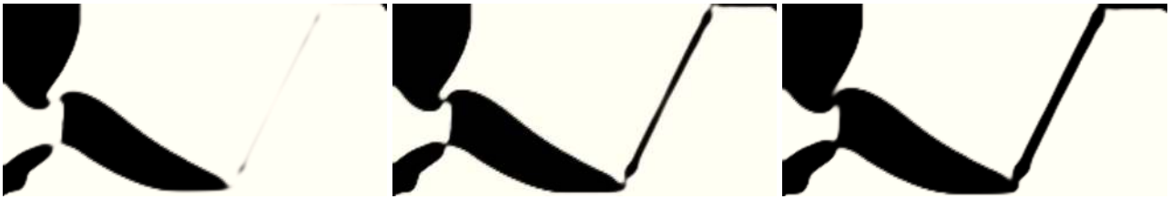
Figure 3. Three threshold projections, eroded, intermediate and dilated, obtained with thresholds \eta = 0.6, 0.5 and \eta = 0.4 , respectively. The design is obtained using large displacements deterministic optimisation formulation with threshold \eta = 0.5 and volume constraint 30% of the original volume imposed on the dilated projection at \eta = 0.3 . The objective is c = -29.12 \mu\text{m} and the projection parameter is \beta = 32 .
