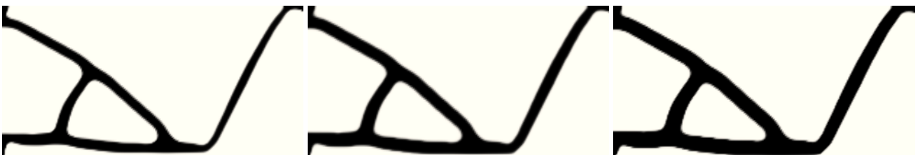
Figure 6. Three threshold projections, eroded, intermediate and dilated, obtained with thresholds \eta = 0.6, 0.5 and \eta = 0.4 , respectively. The design is obtained using large displacements robust optimisation formulation with threshold \eta \in \mathcal{U}[0.2, 0.8] and volume constraint 30% of the original volume imposed on the dilated projection at \eta = 0.2 . The objective is E[c] = -6.12 \mu\text{m} , the standard deviation is \text{STD}[c] = 4.00 , the number of the integration points is 31, and the projection parameter is \beta = 32 .
