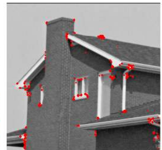
Figure 7. Corners detected from real imagery
