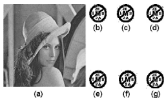
Fig.11 a) Digital watermarking image add Salt & Pepper noise. b) Extracted watermark for proposed method set of the LSB 1 c) Extracted watermark for proposed method set of the LSB 2 d)
