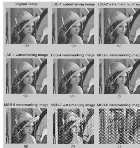
Fig.3 Grayscale images and their 8 corresponding bit planes (from left to right, original images, LSB_1, \dots, and LSB_4 & MSB_5, \dots, and MSB_8 , respectively).
