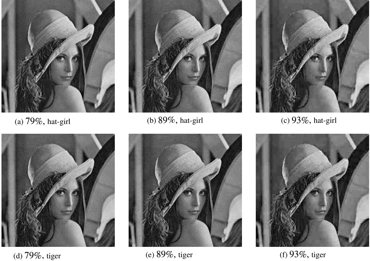
FIGURE 5. JPEG compressed embedded Lena image. The compression factor and the signature image used are indicated below each image. The scale factor used was \alpha = 7 .
