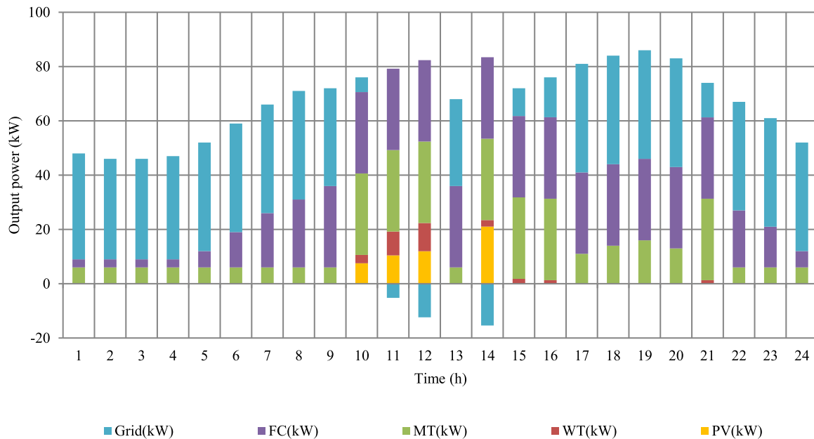
FIGURE 7. Optimal hourly output powers of PV, WT, MT, FC, and utility in the base case.
